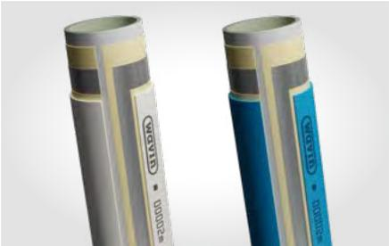
Figure 2: Multilayer pipe for Potable water, heating and air pressure applications (Left) and Multilayer pipe for low temperature installation of heating system (Right)
